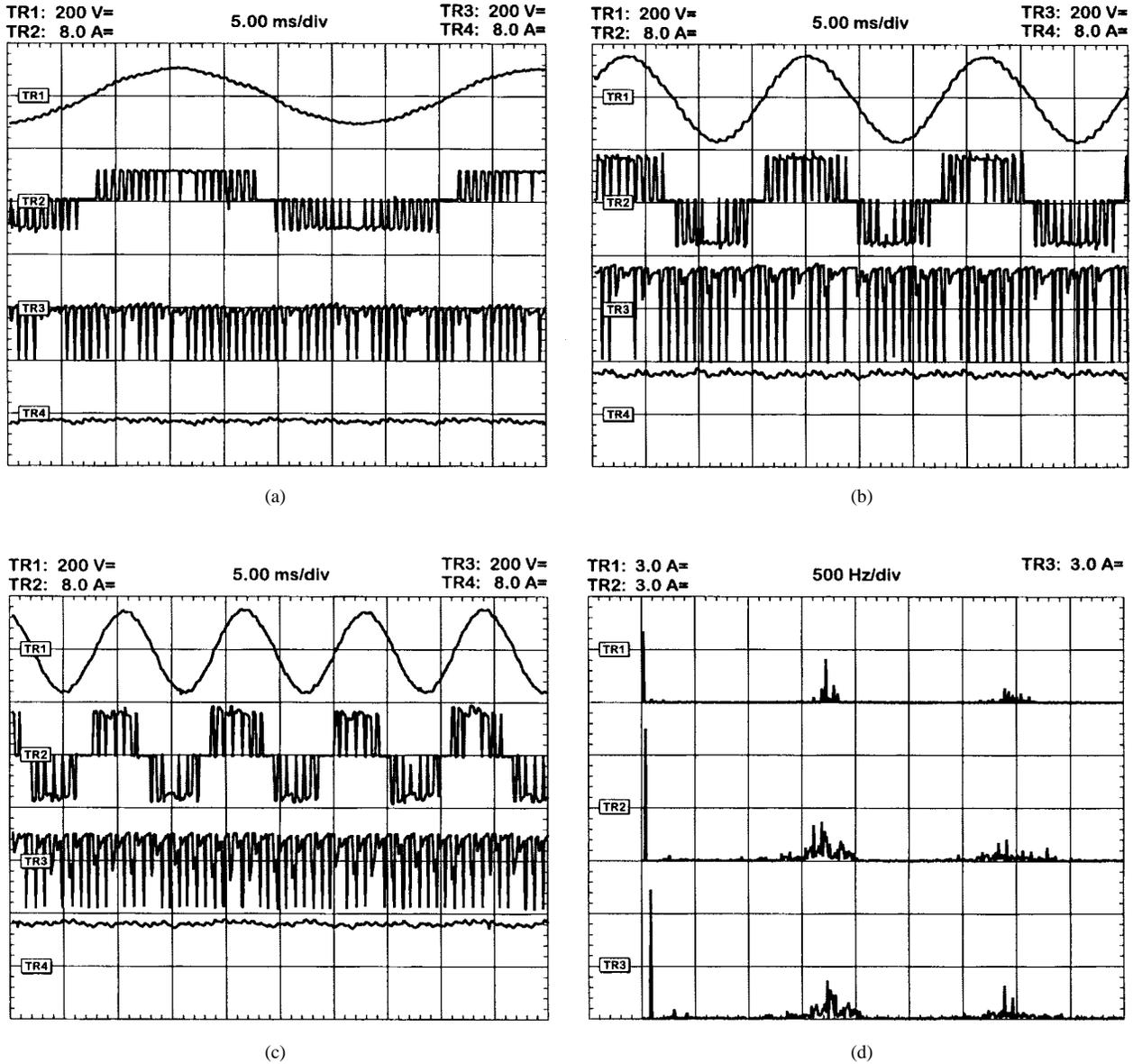
Fig. 4. Experimental waveforms for the proposed CSI-based ac drive. (a) 30-Hz operation. (b) 60-Hz operation. (c) 90-Hz operation. (*TR1*: motor line voltage ( $v_{ab}$ ); *TR2*: CSI line current ( $i_{id}$ ); *TR3*: CSI dc-bus voltage ( $v_i$ ); *TR4*: dc-link current ( $i_{dc}$ )). (d) CSI line current spectrum ( $i_{id}$ ). (*TR1*: 30-Hz operation; *TR2*: 60-Hz operation; *TR3*: 90-Hz operation.)
