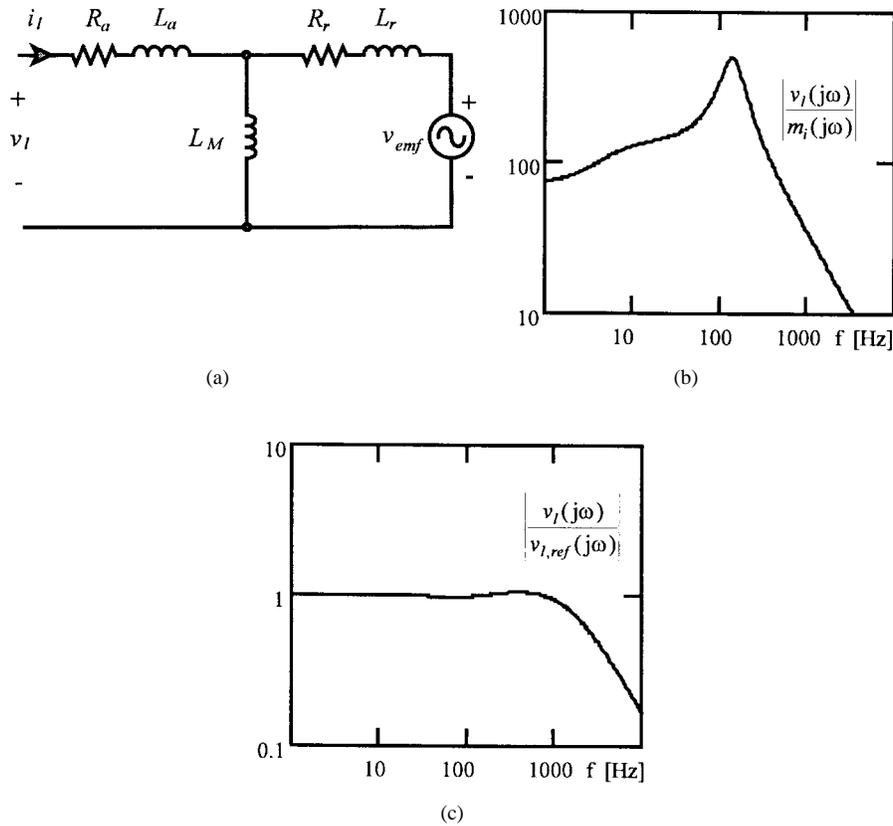
Fig. 8. Transfer functions. (a) Induction machine per-phase equivalent circuit. (b) Motor voltage ( $|v_I|$ ) to modulating waveform ( $|m_i|$ ), open-loop case. (c) Motor voltage ( $|v_I|$ ) to motor voltage reference ( $|v_{I,ref}|$ ), closed-loop case. 3-hp 208-V three-phase 60-Hz motor with  $R_a = 0.6 \Omega$ ,  $R_r = 0.6 \Omega$ ,  $L_a = 2.12$  mH,  $L_r = 2.12$  mH,  $L_M = 53$  mH; converter parameters:  $C_i = 100 \mu\text{F}$ ,  $I_{dc} = 10$  A,  $k_{vl} = 0.5$ ,  $T_{vl} = 1$  ms.
