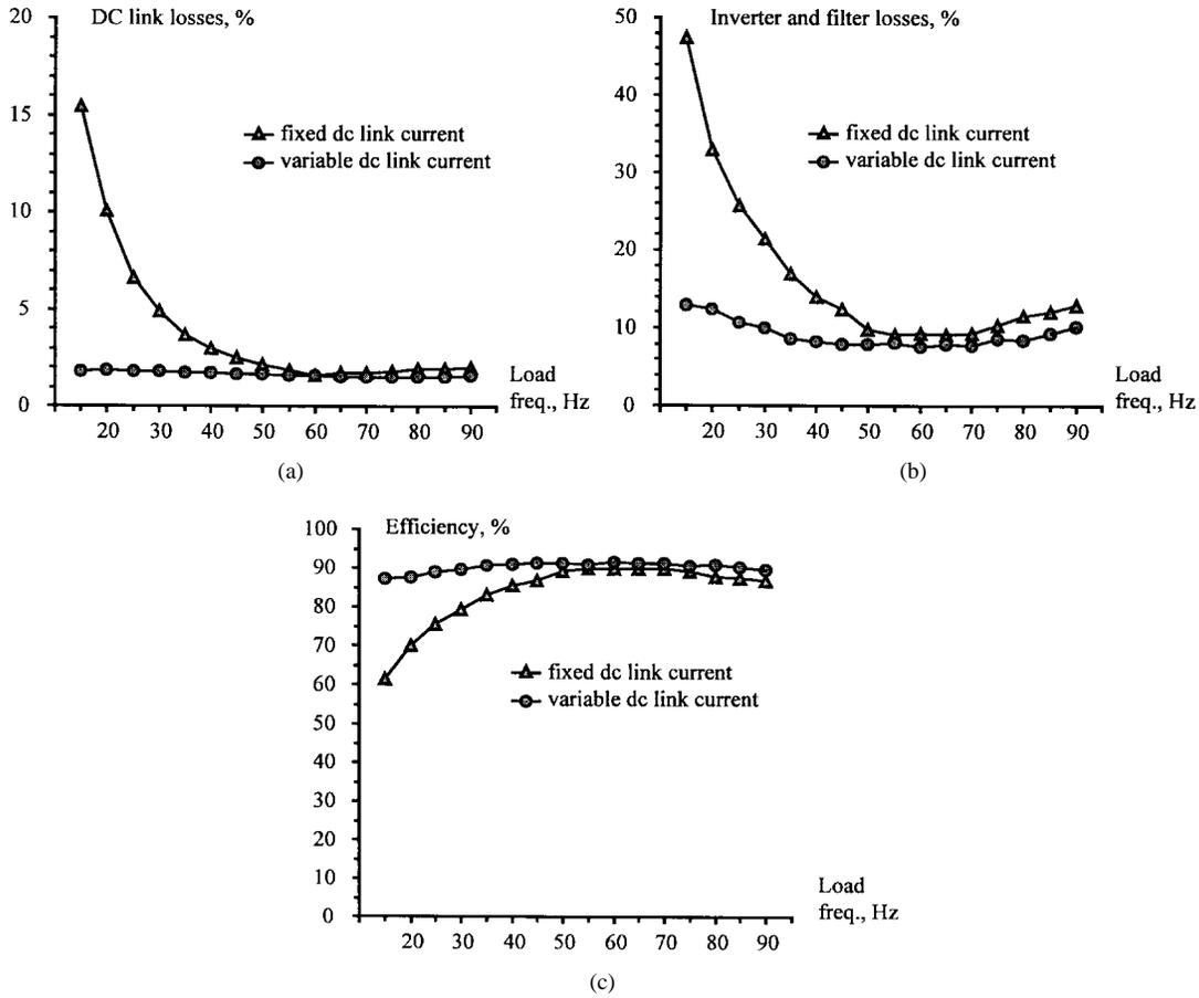
Fig. 7. DC-link and output stage losses as a function of the load frequency (speed). (a) DC-link inductor losses. (b) Inverter and output filter losses. (c) Inverter stage efficiency (including the filter capacitor and dc-link inductor) (experimental results for a sampling frequency  $f_{\text{sample}} = 1.8$  kHz, filter capacitor  $X_{C_i} = 4$  pu, and dc link inductor  $X_{L_{dc}} = 2$  pu).
