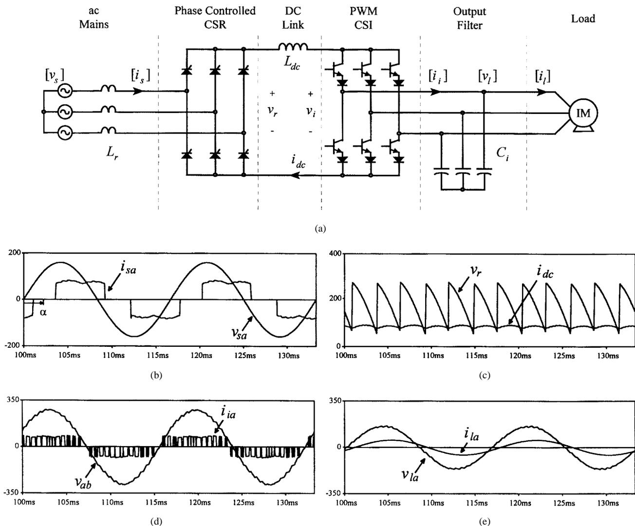
Fig. 1. AC drive CSI based on a phase-controlled front-end rectifier (50% nominal load and 60-Hz output). (a) Power topology. (b) Supply phase voltage ( $v_{sa}$ ) and supply line current ( $15 \cdot i_{sa}$ ). (c) DC rectifier voltage ( $v_r$ ) and dc-link current ( $15 \cdot i_{dc}$ ). (d) CSI line current ( $i_{ia}$ ) and load line voltage ( $v_{ab}$ ). (e) Load phase voltage ( $v_{la}$ ) and load line current ( $15 \cdot i_{la}$ ).
