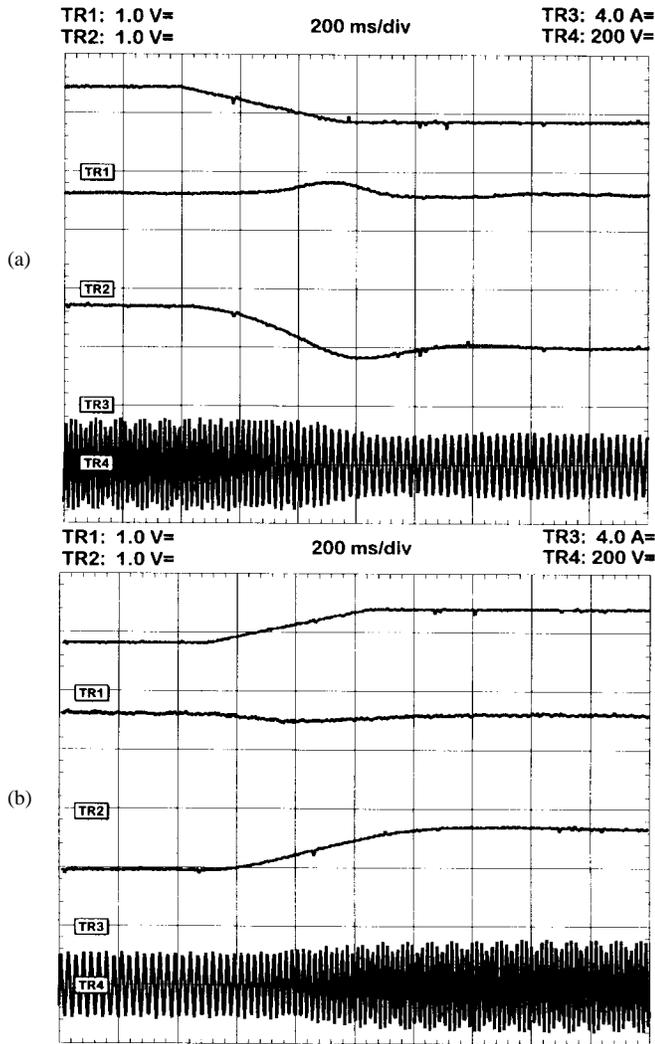
Fig. 5. Experimental transient responses to speed reference changes of the CSI drive based on variable dc-link current operation mode. (a) Ramp decrease from 60 to 40 Hz. (b) Ramp increase from 40 to 60 Hz. (*TR1*: normalized motor speed command ( $\omega_{m,ref}$ ); *TR2*: CSI modulation index ( $m_i$ ); *TR3*: dc-link current ( $i_{dc}$ ); *TR4*: motor voltage ( $v_{ab}$ )).
