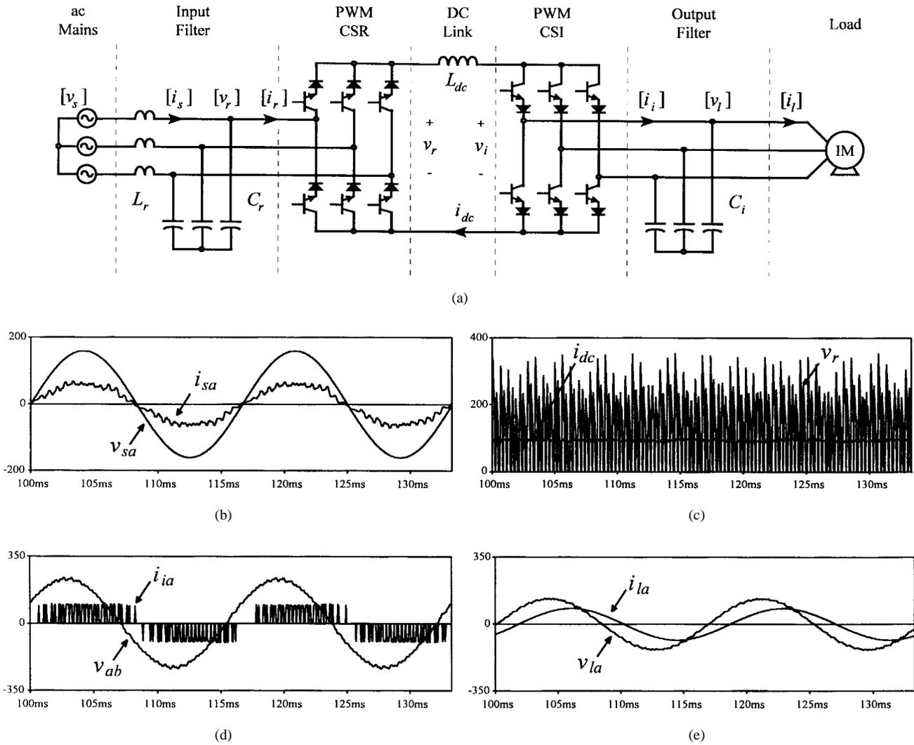
Fig. 2. AC drive CSI based on a PWM front-end rectifier (50% nominal load and 60-Hz output). (a) Power topology. (b) Supply phase voltage ( $v_{sa}$ ) and supply line current ( $15 \cdot i_{sa}$ ). (c) DC rectifier voltage ( $v_r$ ) and dc-link current ( $15 \cdot i_{dc}$ ). (d) CSI line current ( $i_{ia}$ ) and load line voltage ( $v_{ab}$ ). (e) Load phase voltage ( $v_{la}$ ) and load line current ( $15 \cdot i_{ia}$ ).
