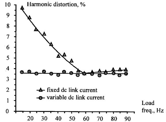
Fig. 6. Motor voltage harmonic distortion ( $THD_v$ ) as a function of the load frequency (speed) (experimental results for a sampling frequency  $f_{sample} = 1.8$  kHz, filter capacitor  $X_{Ci} = 4$  pu, and dc-link inductor  $X_{Ldc} = 2$  pu).
